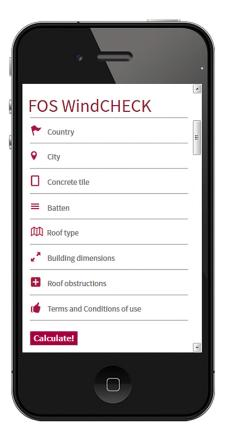
To calculate the clip quantity precisely, its now possible to include roof obstructions such as dormer windows, chimneys etc into the calculation. This has two advantages: the fixing specification shows how to secure the tiles around the obstruction and the clip quantity is automatically reduced by the area of the obstruction e.g. skylights.
