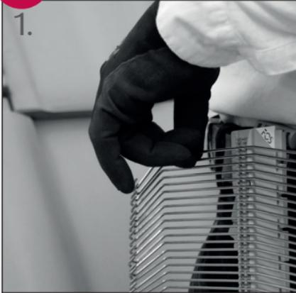
1. Installation time is reduced by up to 25% while using the FOS ClipHOLSTER. Remove clip from the collated strip.
