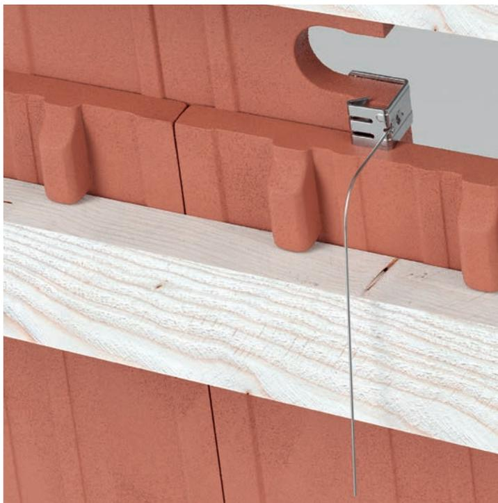
Further the 513 can be used as a replacement lug. The 513 is hammered-in on the side so that the tile has a hold on the batten or sub-construction.
